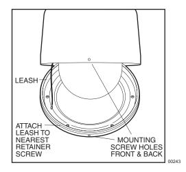
Figure 2. Lower Dome Installation, Pendant Models
